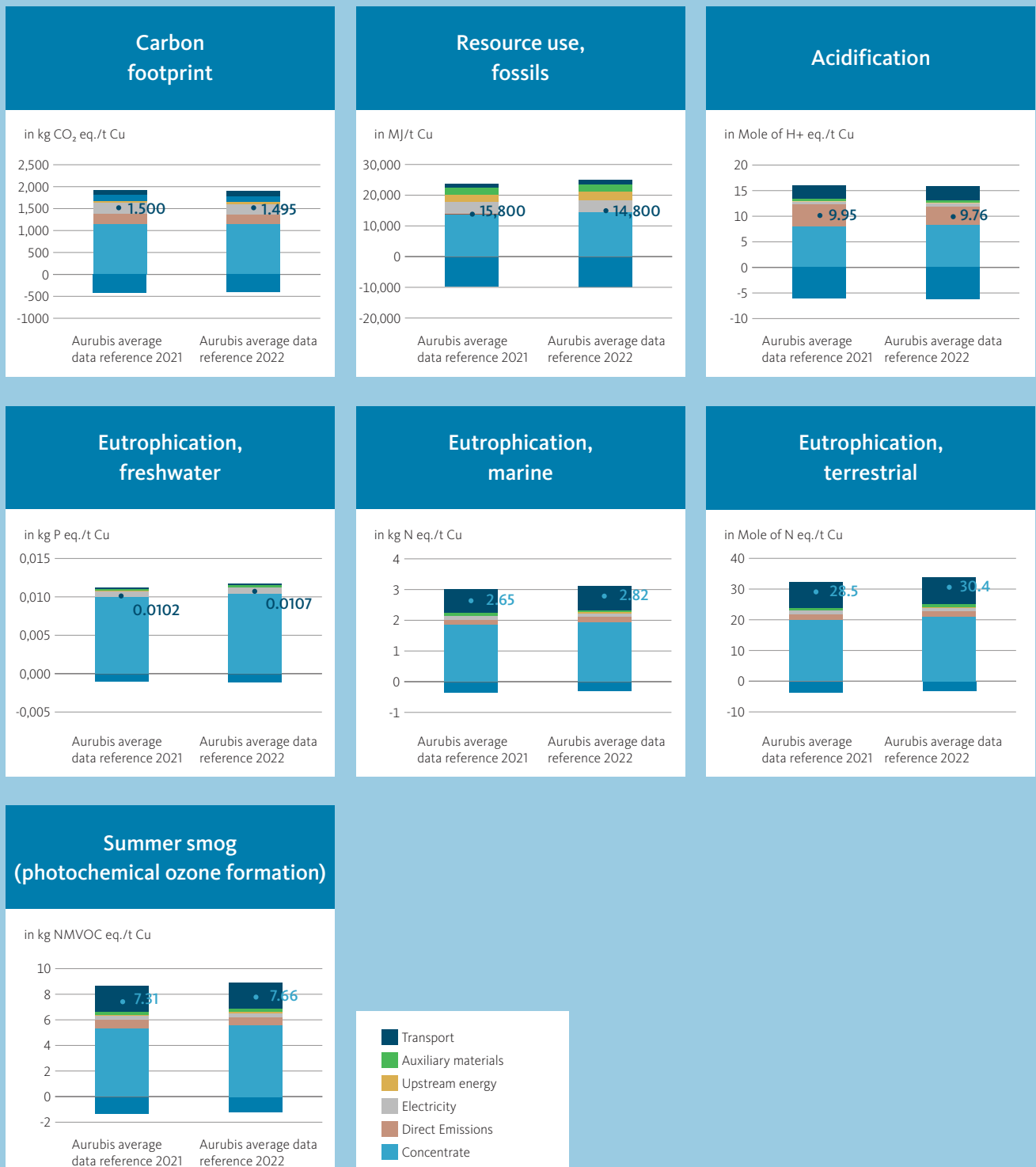
Figure 1: Results for 1 ton of Aurubis average copper cathode (2021) and (2022), (Environmental footprint EF 3.0)
